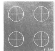
The part and shim must be clean and dry before application. Place the QQI flawside-down in intimate contact with the part being investigated and securely fasten it down on all four sides. To attach the QQIs, use non-fluorescent tape (for example, Scotch brand 191, 471 or 600 series), a strong permanent adhesive such as cyanoacrylate (Super Glue or equivalent), or the Magnaflux supplied test shim stickers. The latter may be removed by soaking in acetone.
