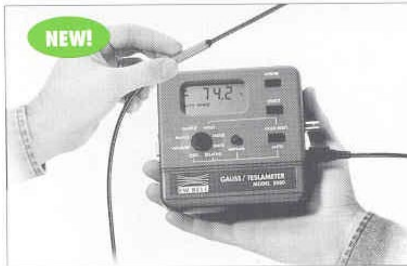
(Fig. 1.1) – Hall Effect Gauss meter (Magnaflux P/N 521043)
