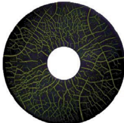
Test liquid spent; time to replace
